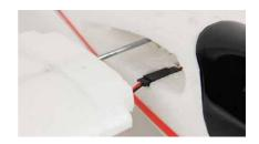
Push the right-hand wing panel fully into the fuselage, preceded by the aileron servo lead as before. Be sure to maintain the dihedral otherwise some difficulty may be experienced in getting the wing to fit.
