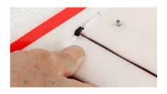
Turn the Alpine upside-down and tighten the wing fixing screws to lock the panels in position. Give the panels a gentle tug to ensure they're secure.
