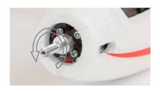
Unplug the LiPo battery and switch OFF the transmitter. Re-assemble the propeller and spinner making sure to tightly secure the propeller nut before refitting the spinner cone.
