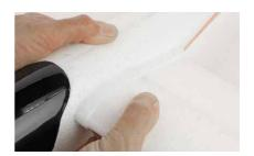
4. Take the steel wing spar and with the bend facing upwards forming a shallow V-shape (dihedral), slide it through the fuselage and fully into the left-hand wing panel.
