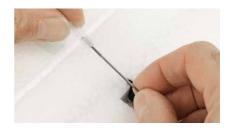
16. Make sure the control surfaces operate in the correct direction noting the following recommended control movements:
